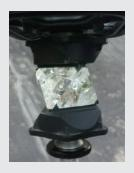
Since most common prisms are bonded together, if one piece of glass breaks, all the glass will need to be replaced.
